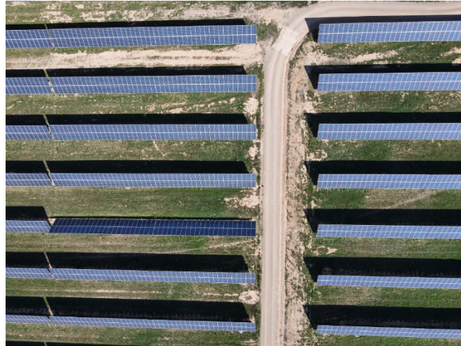
Figure 24. Misaligned tracker in a solar farm
