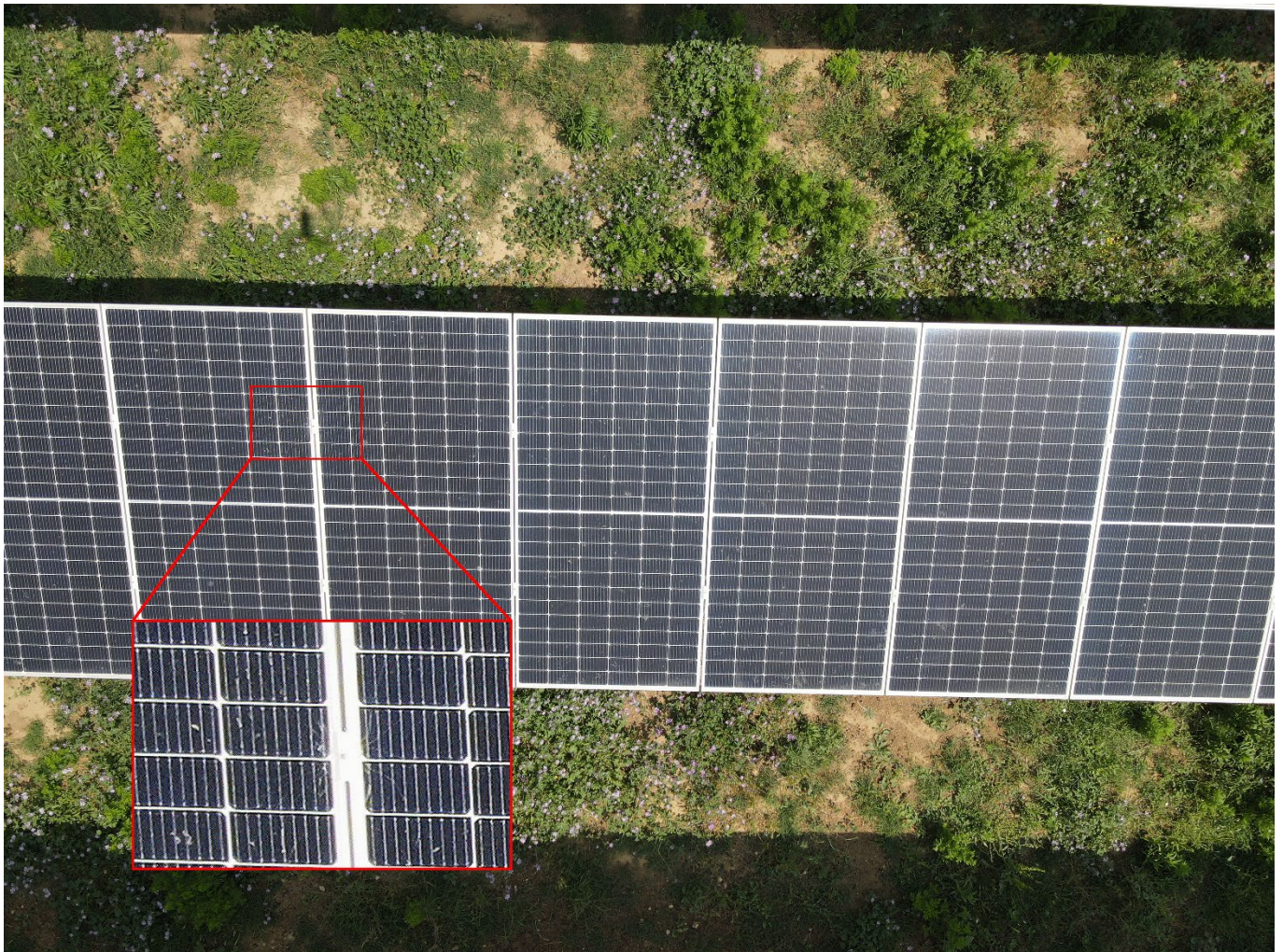
Figure 18. Broken glass in solar plant
