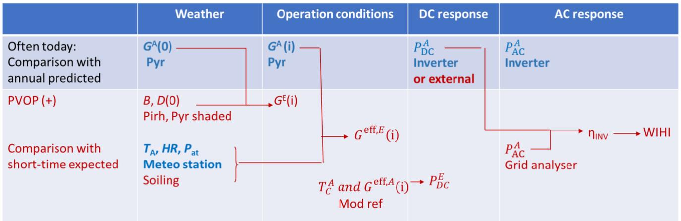
**Figure 2.** Additions required for creating a PVOP digital twin. New variables to be measured appear [ $B$  and  $D(0)$ ], respectively, meaning normal direct and horizontal diffuse irradiances;  $G^{eff}(i)$  measured by a reference module, which also measure the solar cell temperature,  $T_C^A$ ; arrows represent calculations leading to expected values, signaled by the subscript “E”.
