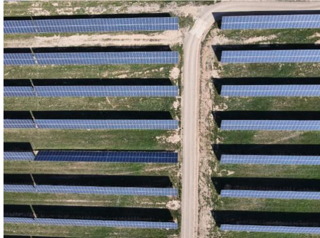
**Figure 12.** Misaligned tracker in a solar farm
