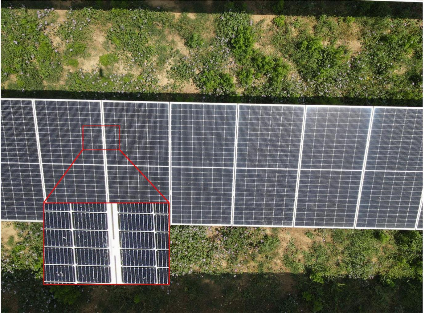
**Figure 6.** Broken glass in solar plant
