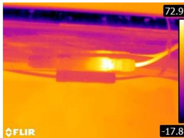
**Figure 14.** Overheated DC connector
